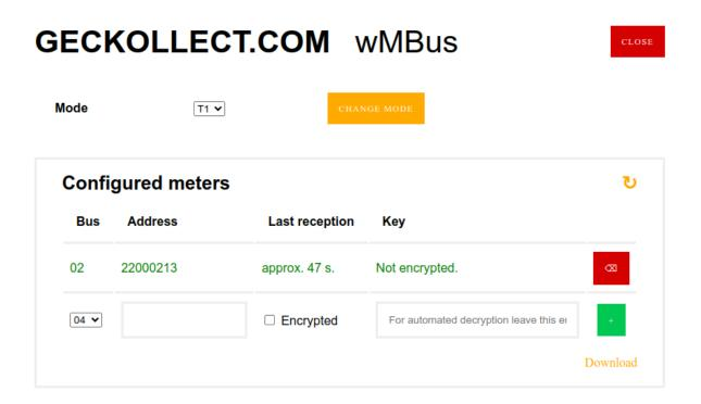
Each meter will respond via modbus on the address associated with it in the column Bus. You should fill the Address field shown on the meter, and tick the Encrypted checkbox if needed.
